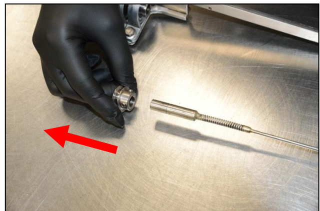
12 - Remove the roller and replace it with a new one.
