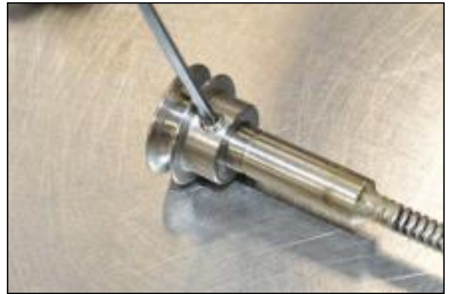
11 - Unscrew the pulley
