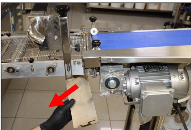
3 - Remove the crumb tray
