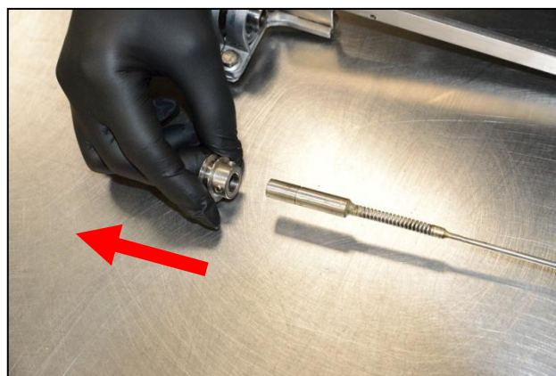
12 - Remove the roller and replace it with a new one. 13 - Reassemble the roller
