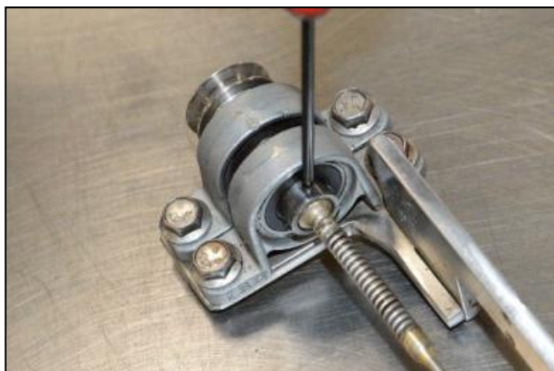
8 - Unscrew the two screws that secure it to the first bearing
