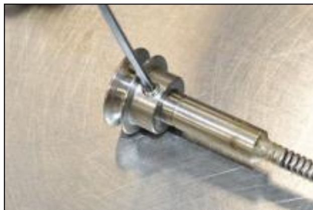
11 - Unscrew the pulley
